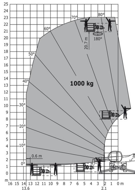
Machine on lowered stabilisers with 3D positive Metric
