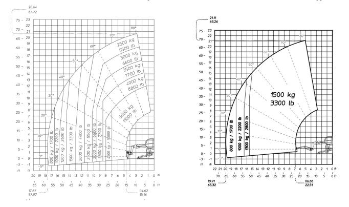
Machine on lowered stabilisers with 365 kg platform Metric Machine on lowered stabilisers with 1000 kg platform Metric
